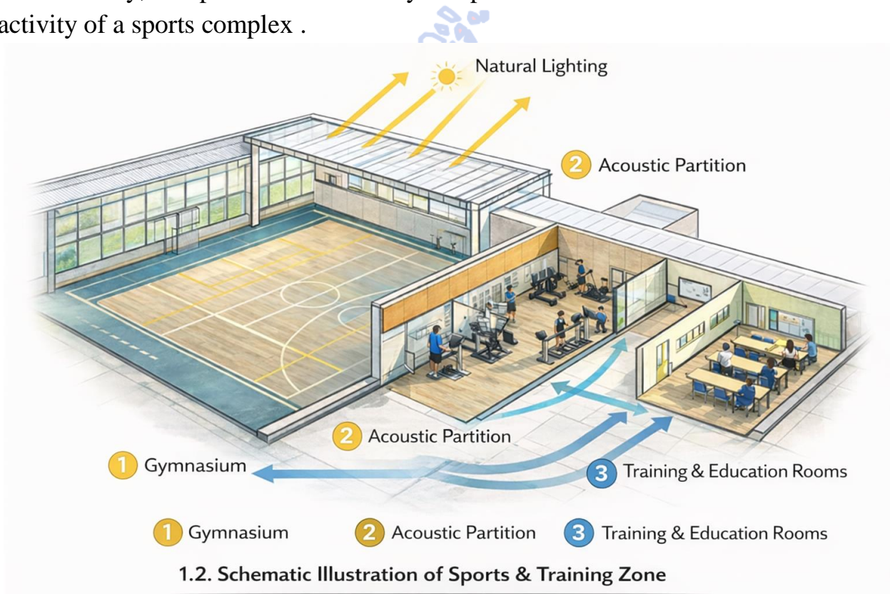
Figure 1. Functional organization of the training and education zone in the sports complex . Training halls and education rooms are located close to the sports activity zone, but partially separated acoustically and functionally, and are provided with natural lighting and ventilation options.
